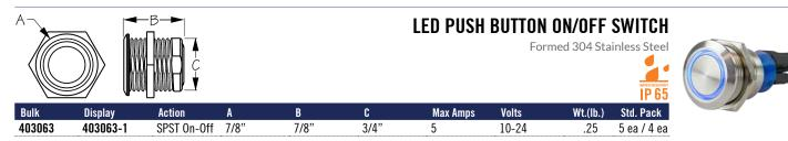
LED Push Button On/Off Switch is prewired for easy installation. Typically wired so LED ring lights up blue when pushing the center button, energizing the circuit. Constructed of corrosion resistant formed 304 stainless steel. 5A max. 10-24VDC. IP65 rating.
