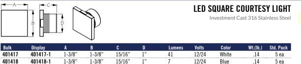
LED Square Courtesy Lights can be mounted to cast light up and down or side to side, depending on the required application. Constructed of corrosion resistant investment cast 316 stainless steel. Installs in a 1" diameter hole; no fasteners required. Available with two white or blue LEDs. 12/24VDC.
