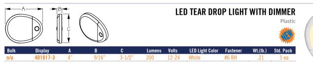
LED Tear Drop Light features a warm white light with blue accented, touch controlled on/dim/off switch. Touch the center button to turn on and off. Continue to touch button to activate dimmer. Warm white, 3000K, 9 Osram LEDs, 200 lumens @ 3W. Works with 12V and 24V systems. Includes two #6 RH fasteners. CE, RoHS compliant.
