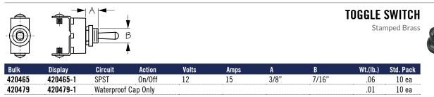
This SPST On/Off Toggle Switch wires easily with two screw terminals. Constructed of stamped brass for durability and corrosion resistance. Maximum panel thickness: 3/8". 15A @ 12VDC. Waterproof Cap (420479) sold separately.
