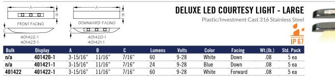
These Large Deluxe LED Courtesy Lights are available with outward or downward directed light. Feature 3 low amp, long life blue or white LEDs with a 60 or 24 lumen output. Constructed of a lightweight plastic body with an investment cast 316 stainless steel cover for a modern, streamlined profile. Installs with two #6 FH fasteners (not included). 9–28VDC. CE compliant. IP67 waterproof rating.
