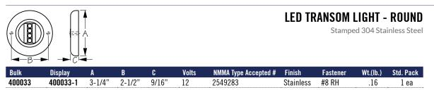
This Round LED Transom Light is approved for USCG 2 NM (Colreg 2 mile). Constructed of corrosion resistant stamped 304 stainless steel. Installs with two #8 RH fasteners (not included).
