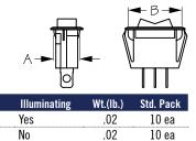
Rocker Switch wires easily with three stamped brass 1/4" blade terminals. Snap-in panel mount fits standard 1-1/8" X 1/2" switch cut-outs. 420441 illuminates red when in the ON position. Constructed of durable weather resistant injection molded nylon and polycarbonate housing. 15A @ 12VDC.
