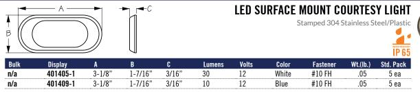
These LED Surface Mount Courtesy Lights utilize three blue or warm white low amp LEDs, providing a very long service life. Constructed of corrosion resistant stamped 304 stainless steel and lightweight plastic. Installs with two #10 FH fasteners (not included). IP65 water resistant rating. 12VDC.
