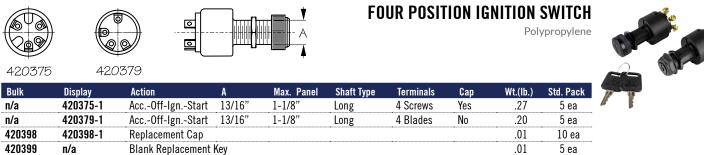
Four Position Ignition Switch for accessory, off, ignition, and start functions. 13/16" diameter long shaft. Maximum panel thickness: 1-1/8". Four screw or four blade terminal electrical configurations. Ignition: 15A @ 12VDC. Solenoid: 30A @ 12VDC. Accessory: 15A @ 12VDC. Constructed of polypropylene. Includes two keys. Screw terminal version includes rubber boot.
