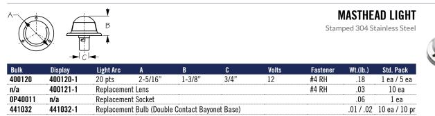
This 225° Masthead Light is for replacement of existing lighting (not for new construction). Constructed of corrosion resistant stamped 304 stainless steel. Installs with three #4 RH fasteners (not included).
