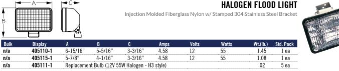
This marine grade Halogen Flood Light features H3 style 12VDC 55W halogen bulb. Constructed of fiberglass reinforced injection molded housing for strength and UV resistance, a solid glass lens, and a corrosion resistant stamped 304 stainless steel mounting bracket.
