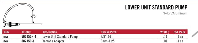
Fits quart oil bottles. Flexible hose gets into hard to reach locations. Threaded (3/8"-16) fitting fits Mercruiser®, OMC®, Evinrude®, Johnson®, Honda® (70hp & up), Volvo®, Force®, Mercury® (US origin models) and Gamefisher® lower units. Includes Yamaha® adapter (8mm-1.25) fitting for Mercury® (Japanese origin models), Yamaha®, Nissan®, Tohatsu®, and Honda®.
