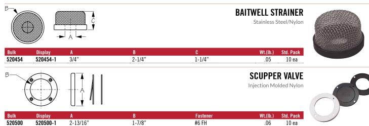
This Scupper Valve provides a water exit for boats with self-bailing cockpits. Ideal for above the water line drainage. Valve features soft black flapper that seals to prevent backwash. Compatible with most self-bailing applications. Constructed of durable injection molded nylon. Surface mounts with four #6 FH fasteners (not included).
