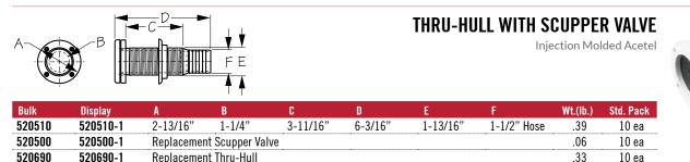
This Thru-Hull Scupper Valve mounts through the transom and provides a water exit for boats with self-bailing cockpits. Ideal for above the water line drainage. Valve features a soft black flapper that seals to prevent backwash. For use with 1-1/2" hose. Compatible with most self-bailing applications. Constructed of injection molded acetal. Installs with four #6 FH fasteners (included).
