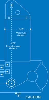
Adjustment of this screw may cause motor failure and void the warranty.
