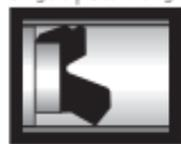
**SHAFT:** The shaft is made of steel with a proprietary hard chromium plating, ground and polished to a smooth non-porous surface for leak-free dynamic sealing.
